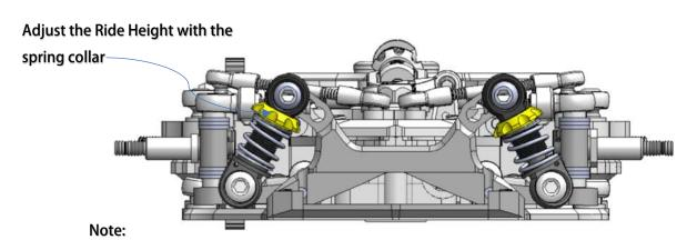
To have a good performance and stable car, the key point is to make sure there is "No droop" no matter what ride height the front it is. That means, the front arm is not able to drop down if you lift the car. Adjust it thru the "droop screw" of the lower arm to achieve this.
