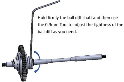
You will see there is wobble between the gear body and the shaft, no worry that is normal and that is on purpose to have this play. We need this play to ensure the system is working smoothly and running quietly with the motor pinion.
